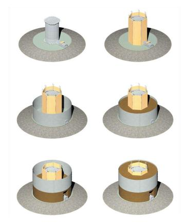
Figure 9. First phases of the silo completion (type B).
